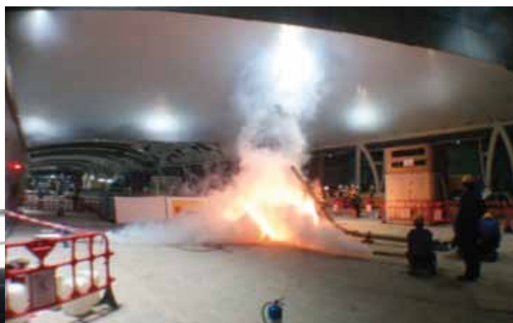
Hot Smoke Test Performed in Midfield Concourse
